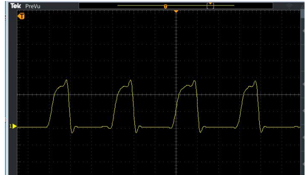
R1 = 10 kΩ pull-up C2 = 680pF 10kHz Switching Magnetic Field
